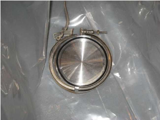
IMG_0441.jpg Removed Blank-off flange
