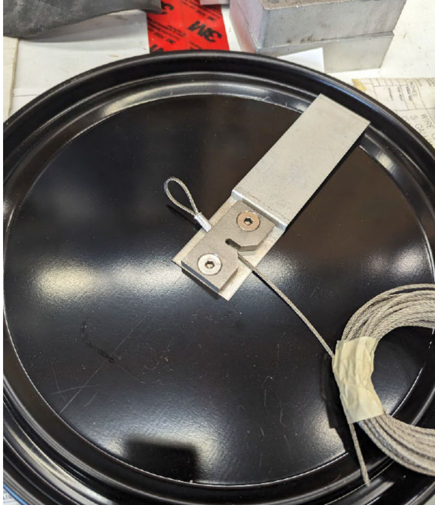
Figure 4: Correct way for cable to be routed through attachment block (example image from TRI-DN-23-10 assembly instructions). For Pail 275, the cable was routed through the block the opposite way.
