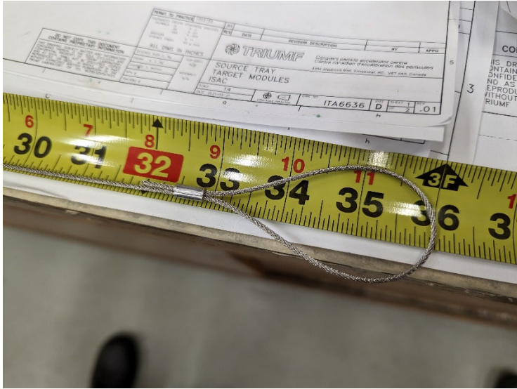
Figure 2: Crimped loop which was added to wire rope (3")
