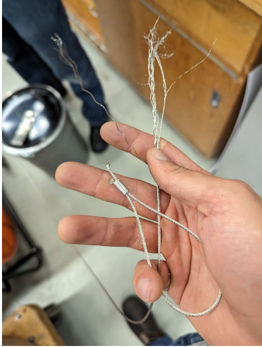
Figure 9: Failure point during intentional destructive testing (beyond what is required for the purposes of this test)
