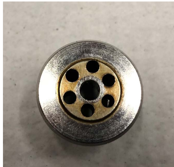
Figure 5: Valve Retainer with material deposit
