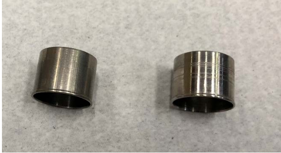
Figure 2: Wear on Face Sleeve (right)
