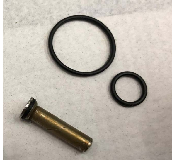
Figure 4: O-rings and valve assembly with O-ring. Valve assembly coated with deposit.
