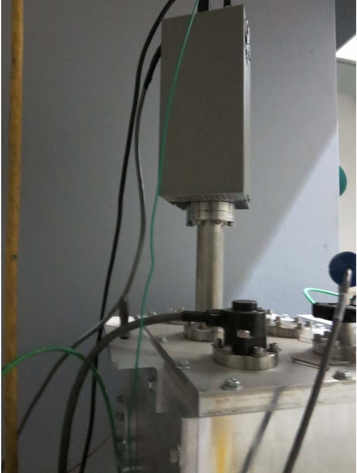
Figure 2: Cable from RGE electronics to diagnostics box
