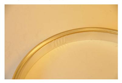
Marked fin with yyyy mm dd on ring with T2 M9 Q1, no drawing/part number.
