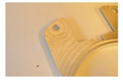
Ring was cleaned in simple green and hot water, wiped dry and packed with indium.
