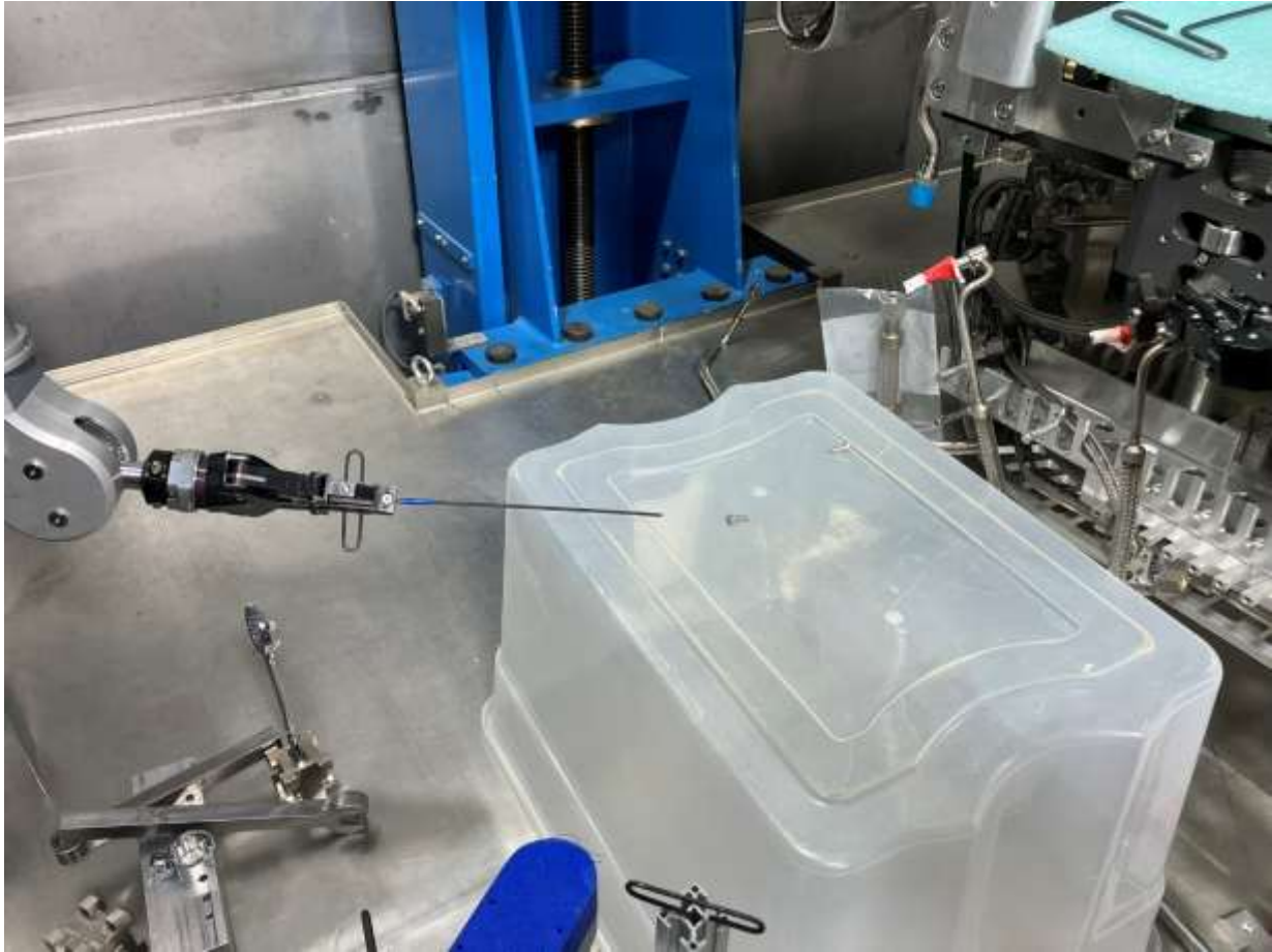
Possible to pick up small shoulder screws with allen key
