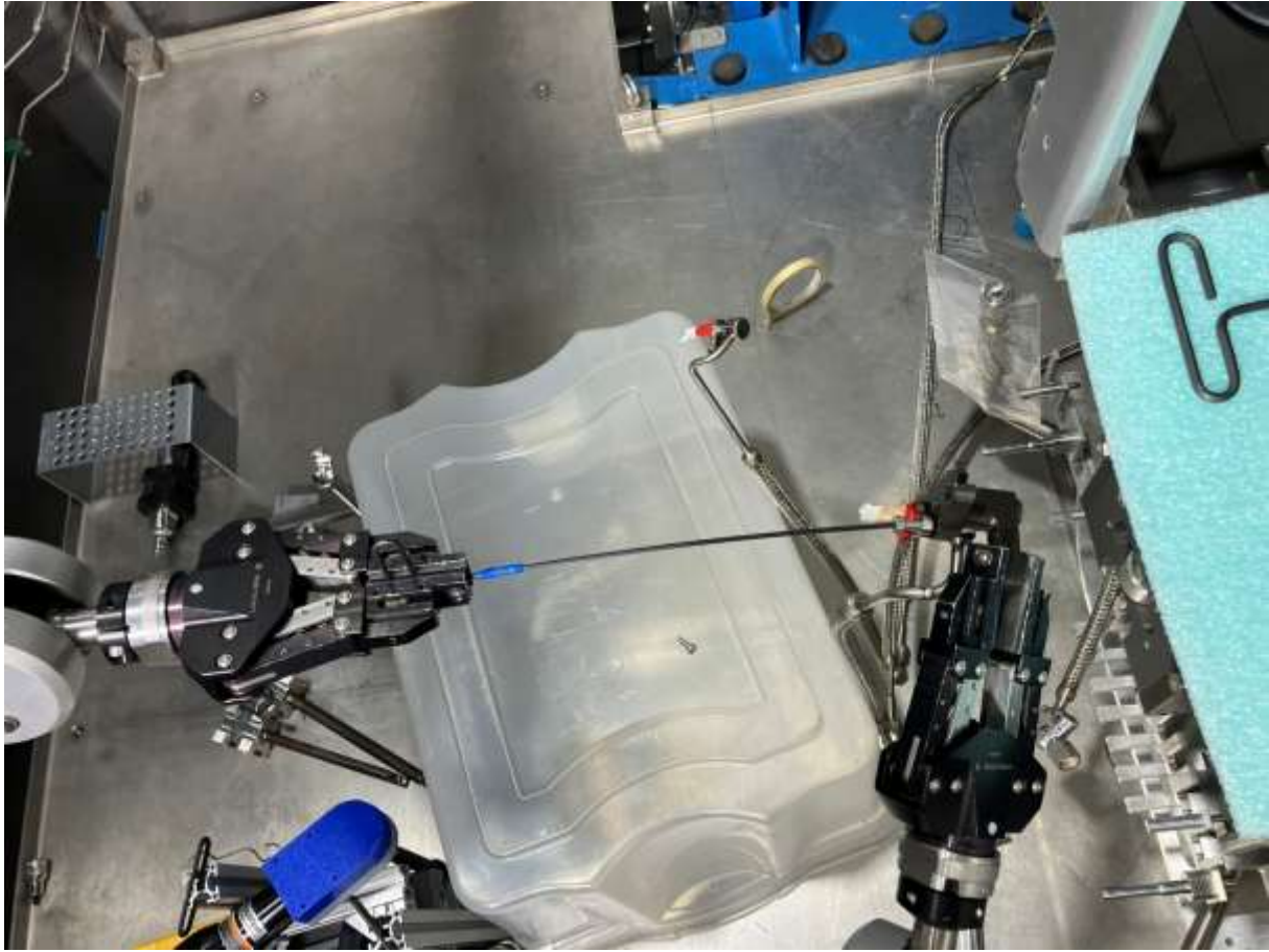
Returning gas lines onto bracket is a 3 manipulator operation.
