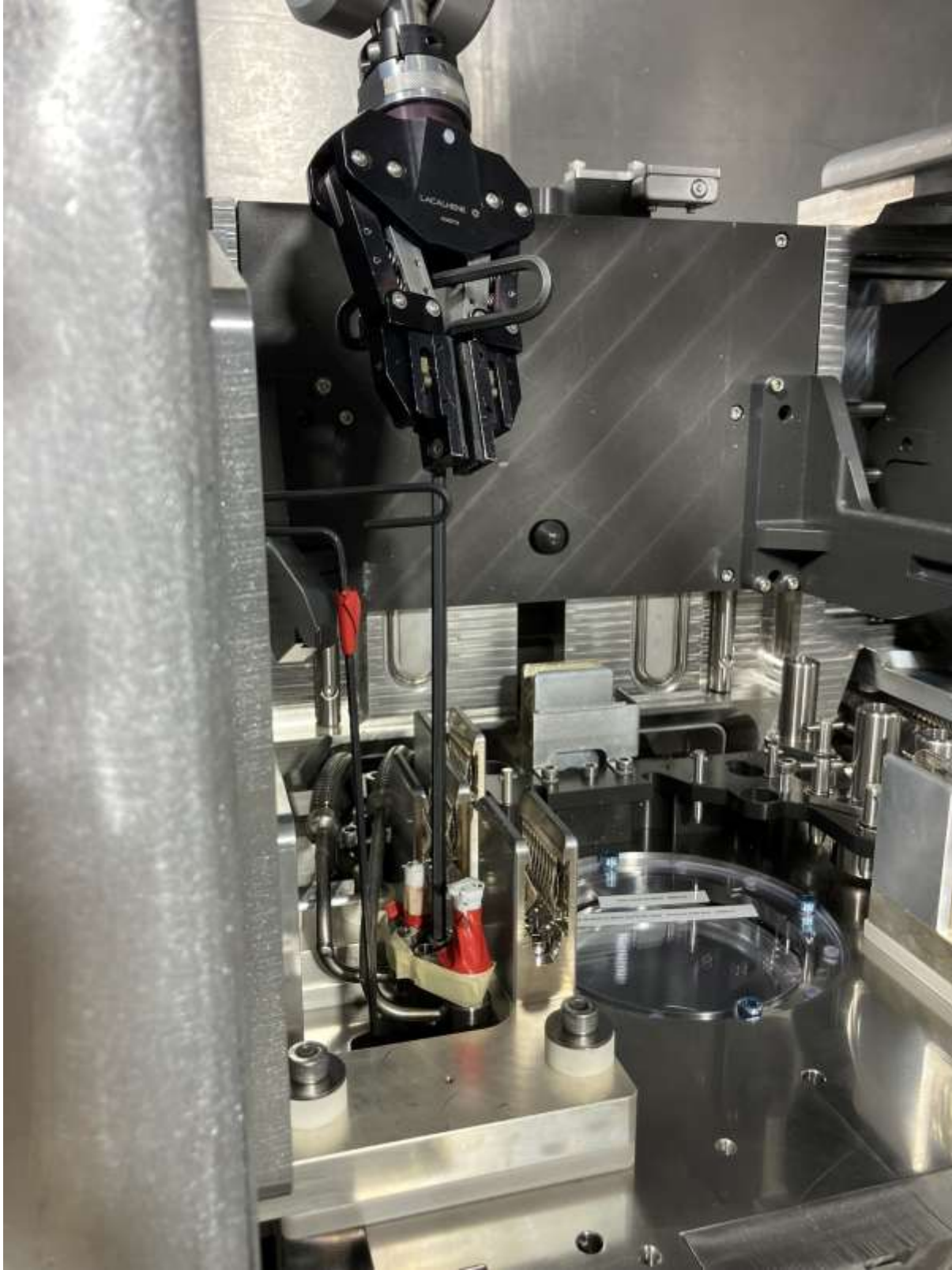
Pinning allen key released to let us turn other allen key for bracket screw
