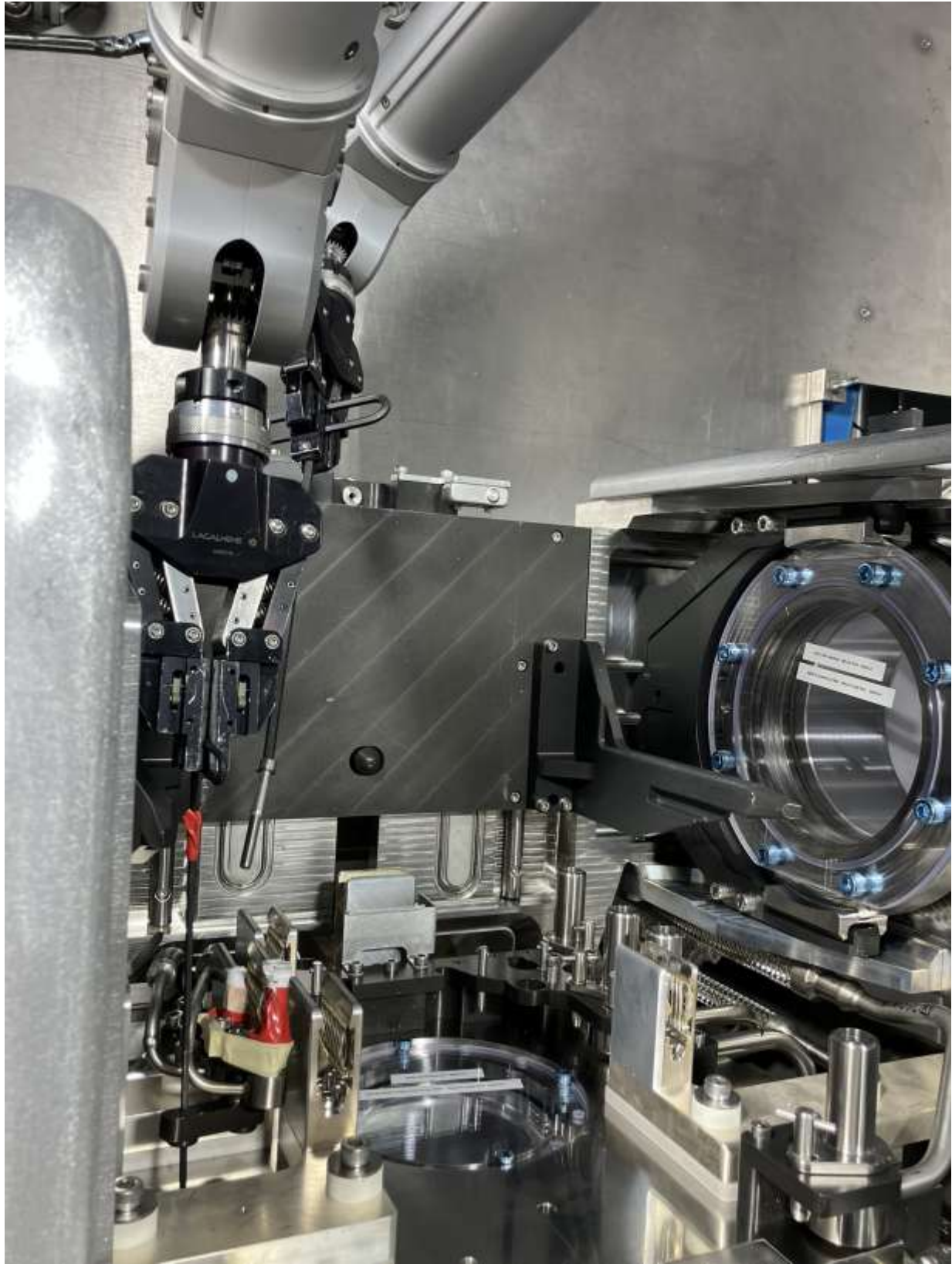
Position of bracket prior to final push onto FE plate with allen key and screw
