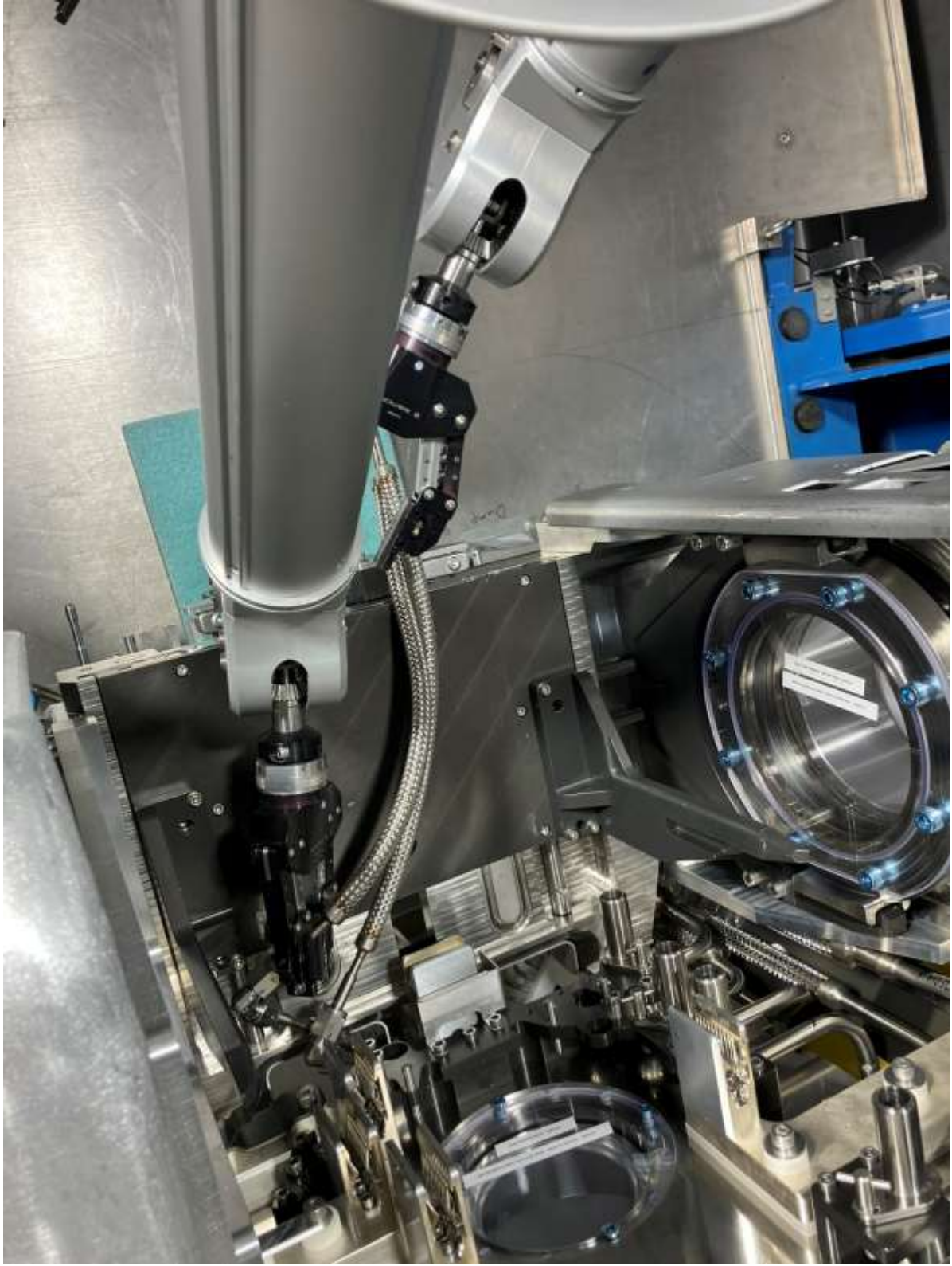
Two manipulator operation to feed in new lines
