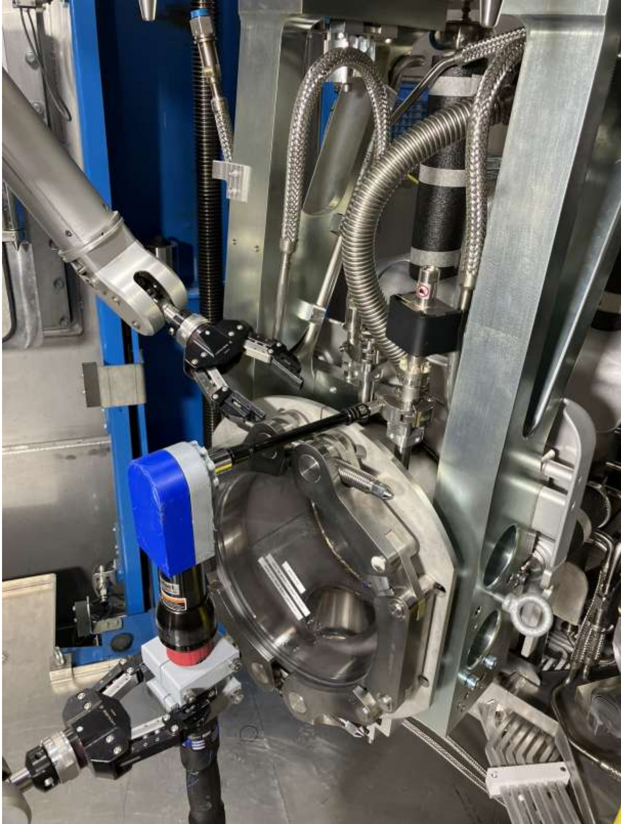
Successfully returned front clamp joint, assuming we have a tool to reinsert the rubber KF gasket.
