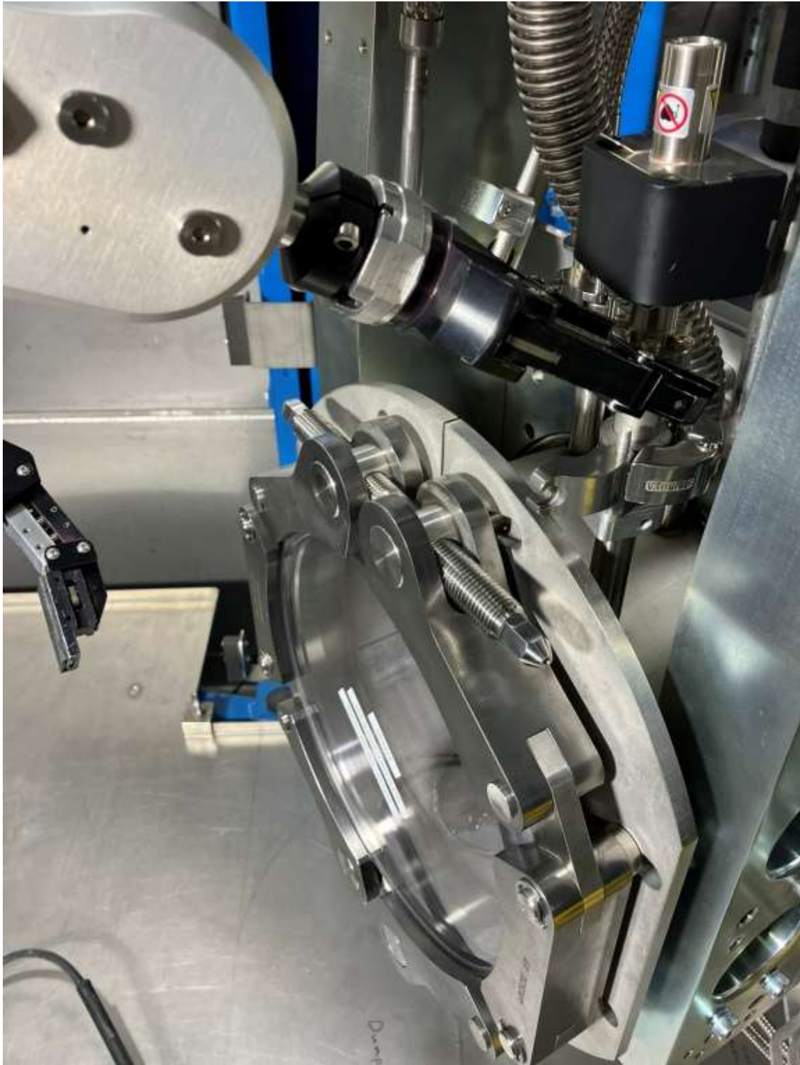
Returning the connector on top of the exterior KF joint.
