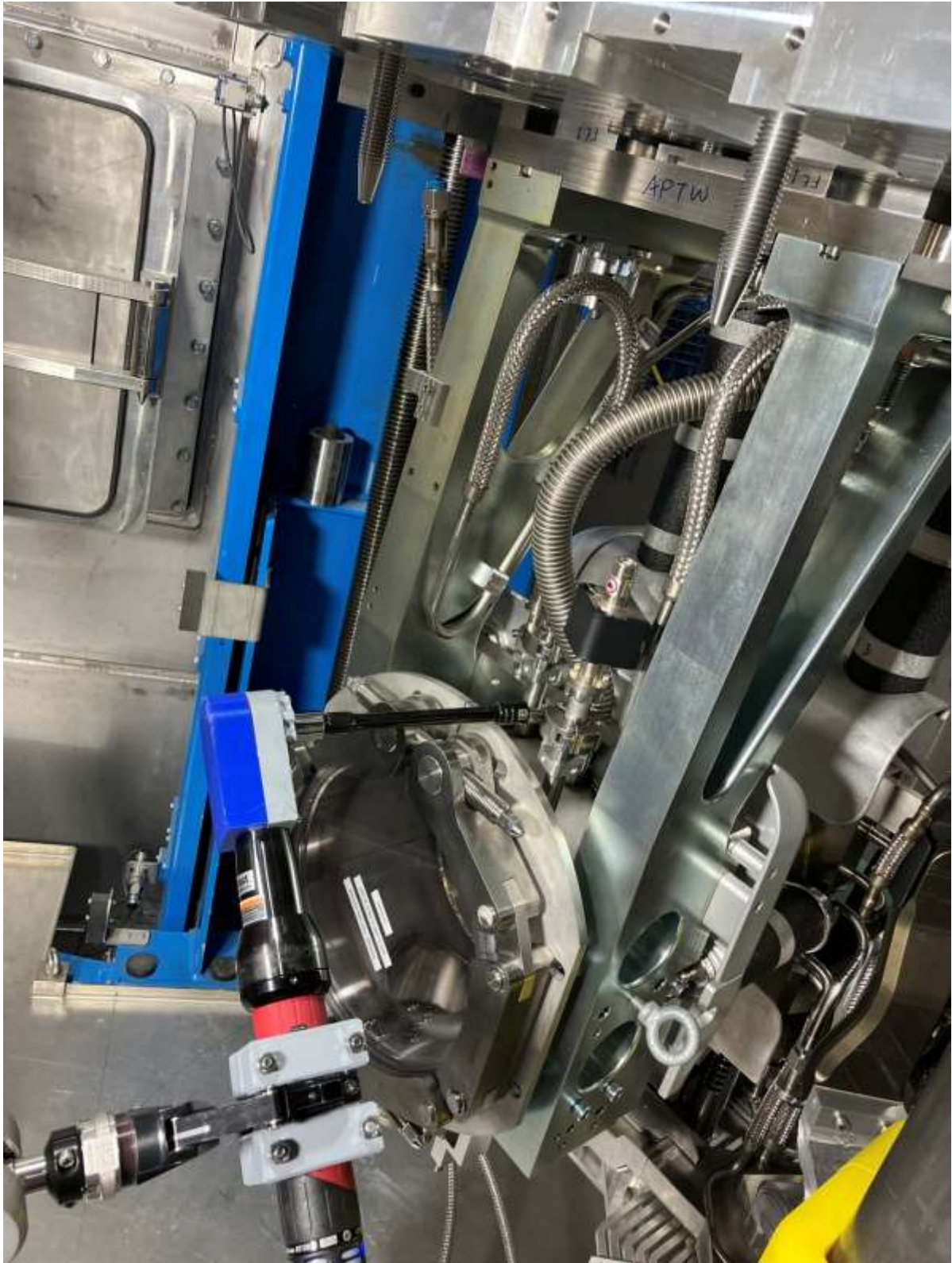
Using torque tool to access nut on clamp. Use only to apply initial torque when undoing, use manipulators to prevent losing nut if not captive.
