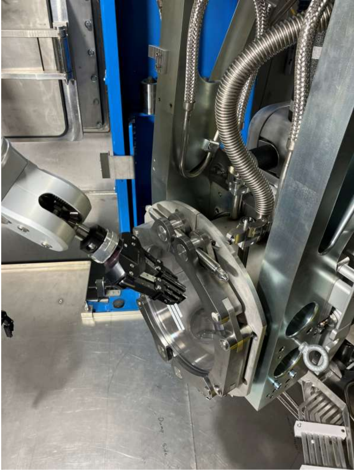
Exterior clamp successfully undone and opened.
