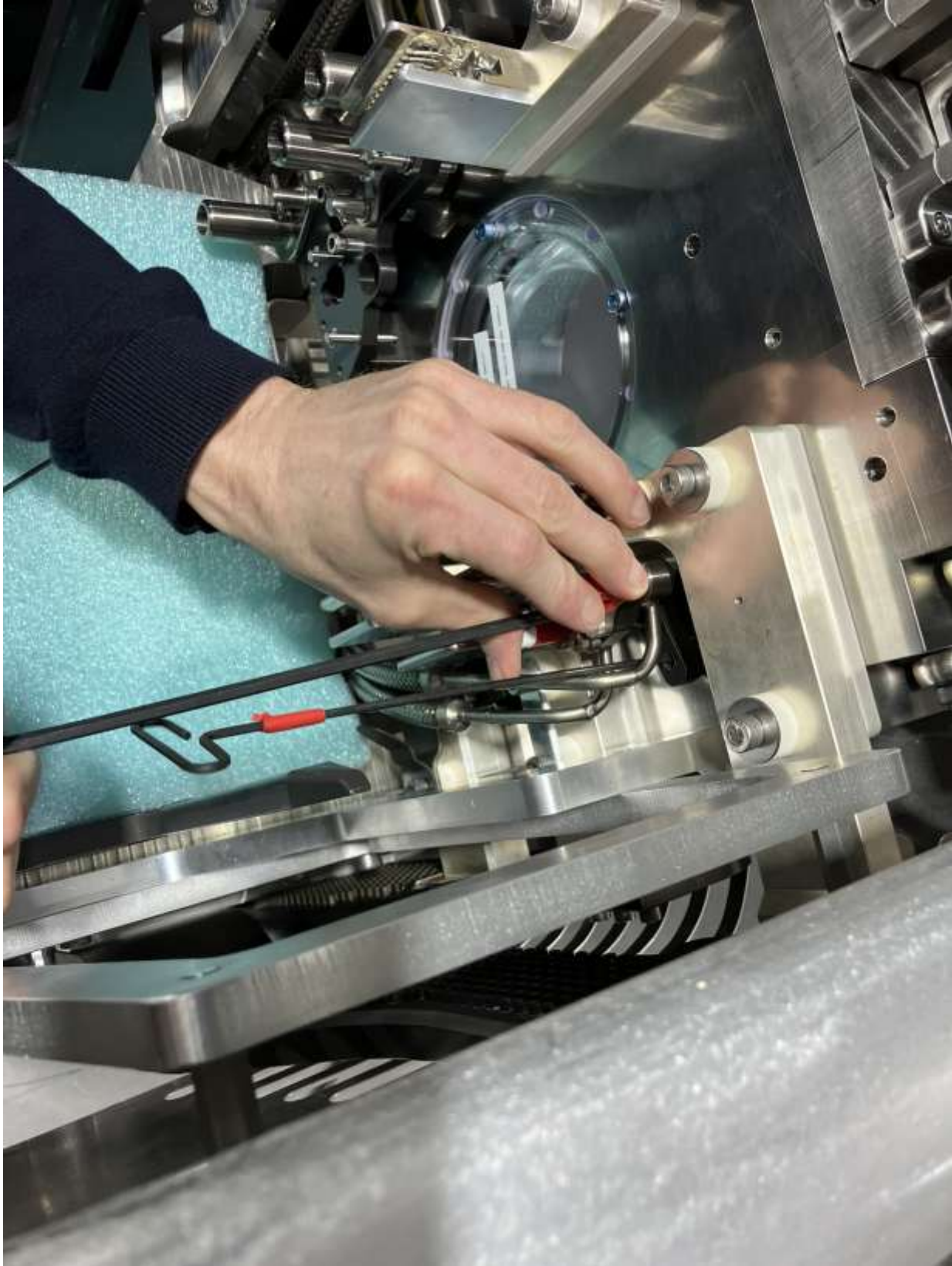
Small Allen key can be used to help guide bracket into location.
