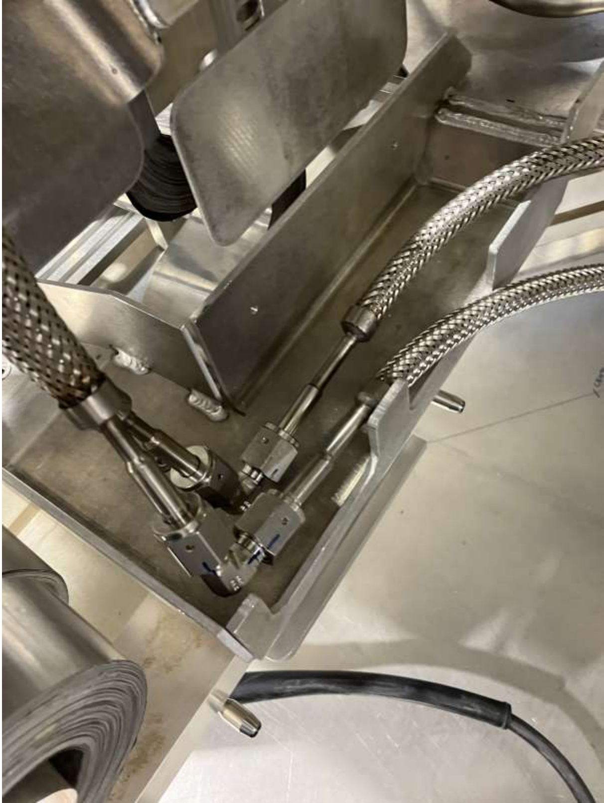
Gas lines have some tendency to 'wedge' in cutouts on the cable guides (see following pictures).
