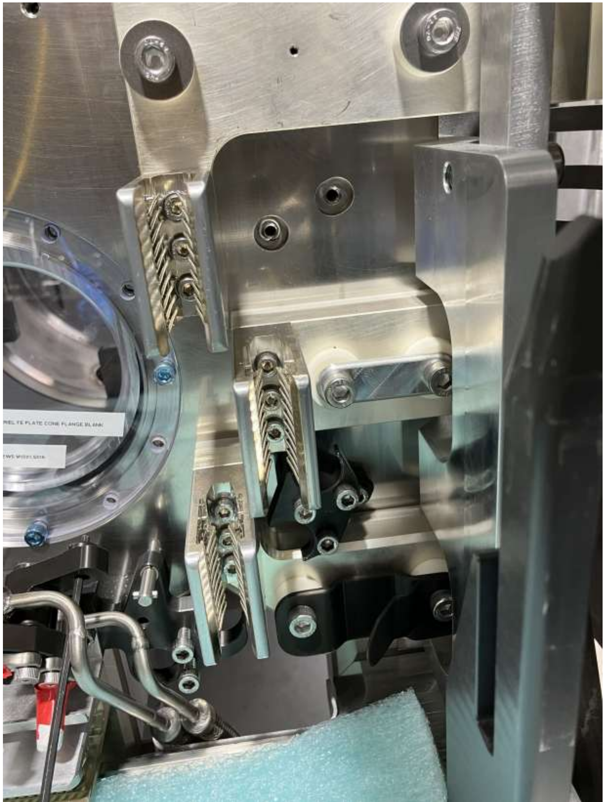
Helicoil insert 'threaded out' and prevents screw on gas line bracket from being re-done.
