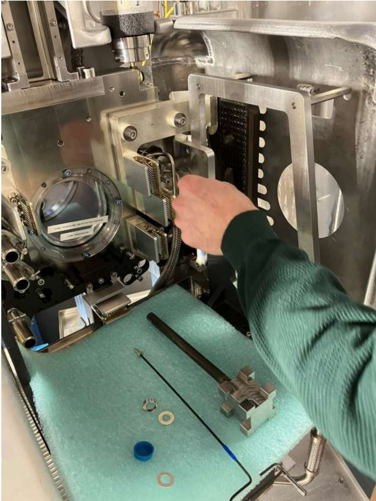
Gas line bracket and screws tested by hand, confident can do if tool is made to grab onto the sealing tube ends without damaging.
