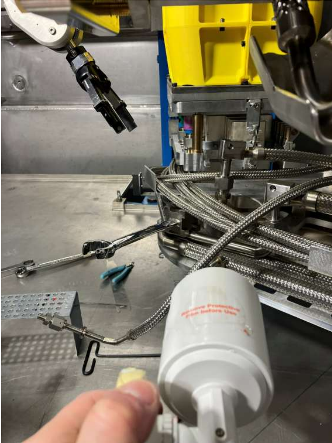
Misalignment not perceived from hot cell window, illustration of possible useful cross-view camera placement.
