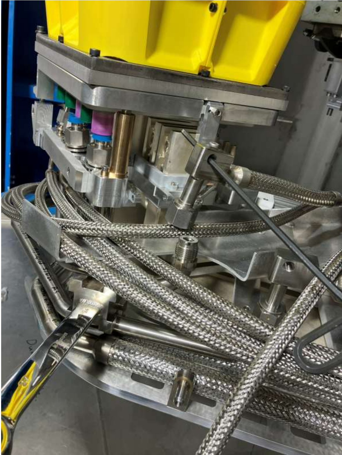
Wrench used to prop up the male side of the line. Using the thru hole on weld body to maneuver the female side into alignment
