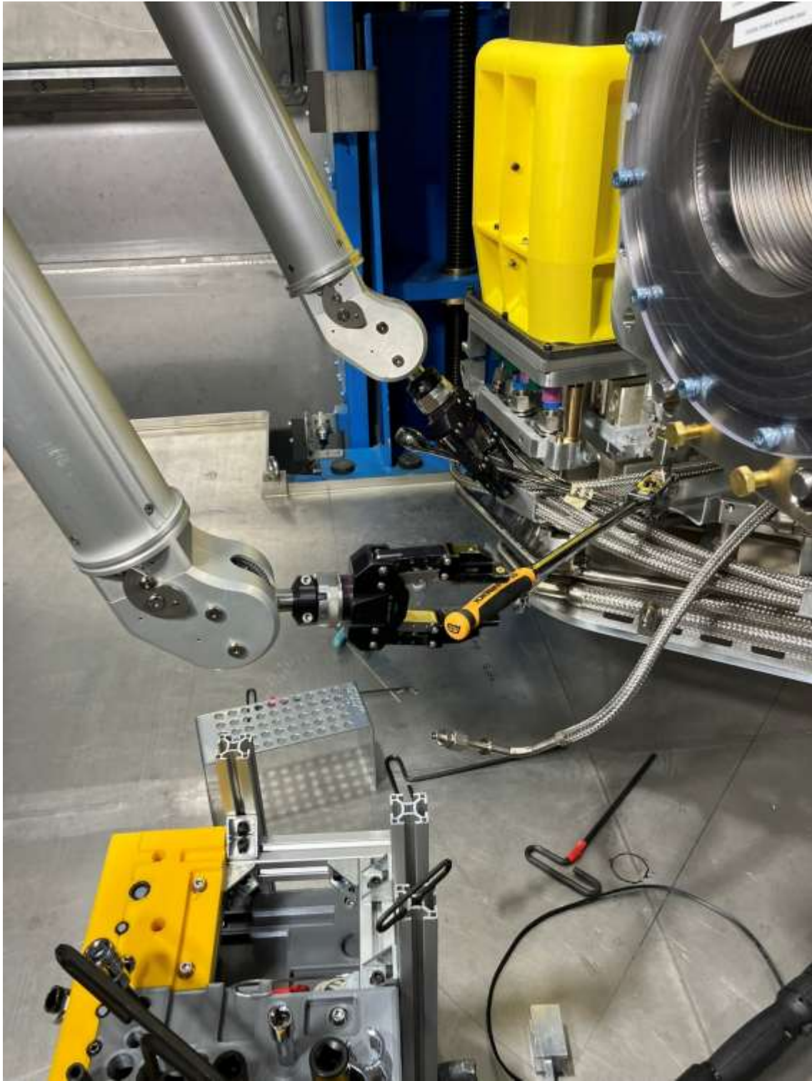
Setup for successful re-establishment of joint. Crows' feet and extra length ratchet used.
