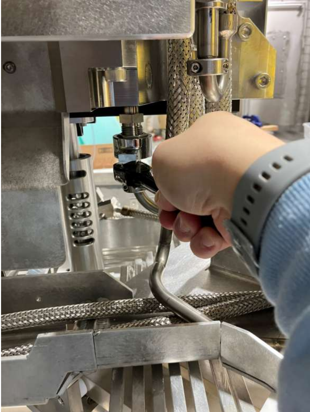
Ratchet and 12-point secure crow's foot wrench can be used in this location for low clearance tightening operations.
