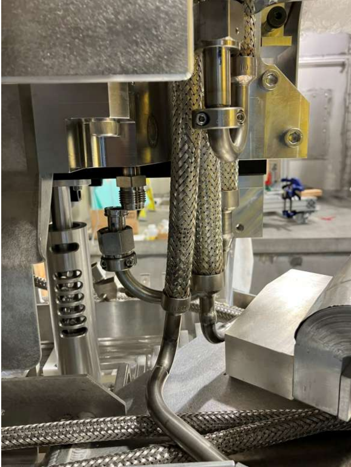
Resting 'misalignment' on this line when not done up. Purchased shaft clamp (McMaster 9648T5) works well to keep the nut from falling too far, also works for u-bend on the second to bottom line. The clamp does not cause the line to catch when being exchanged.
