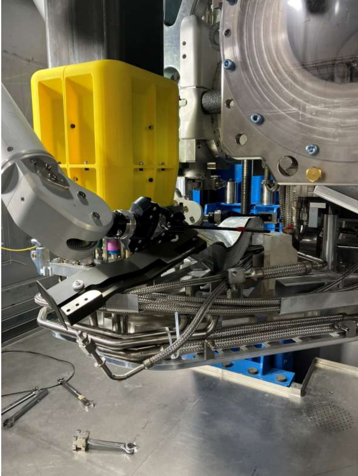
Using hook from one side to position the female VCR side.
