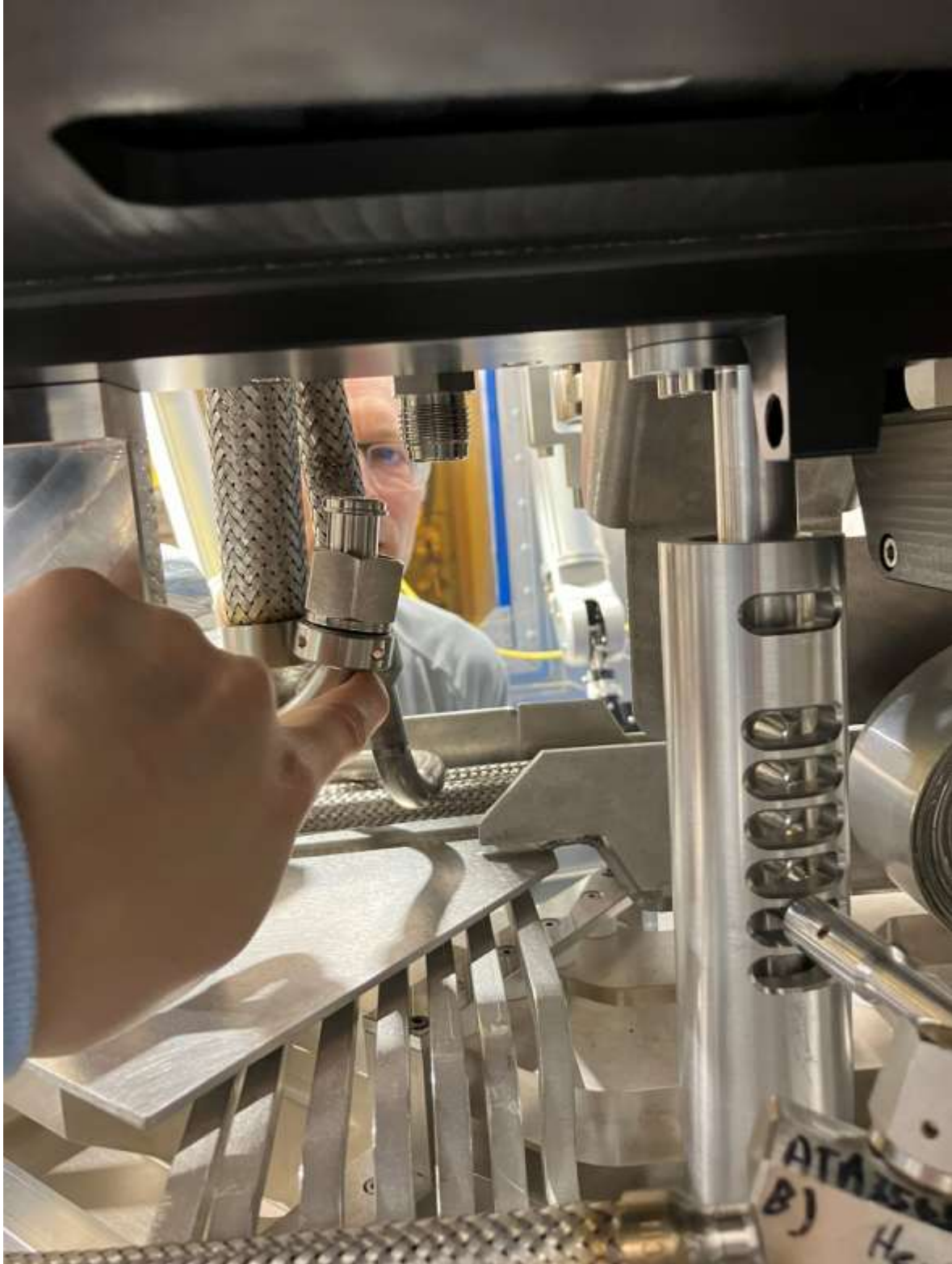
By pushing the flexible line out of the way (pin still attached at dynamic PEEK seal face), we have enough access to insert a VCR gasket to the fixed male VCR.
