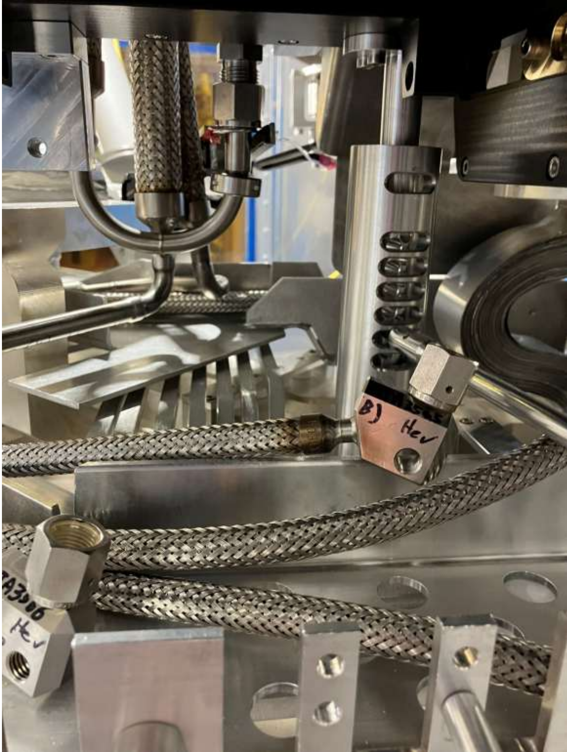
Cramped space when trying to re-start the nut with the starter tool.
