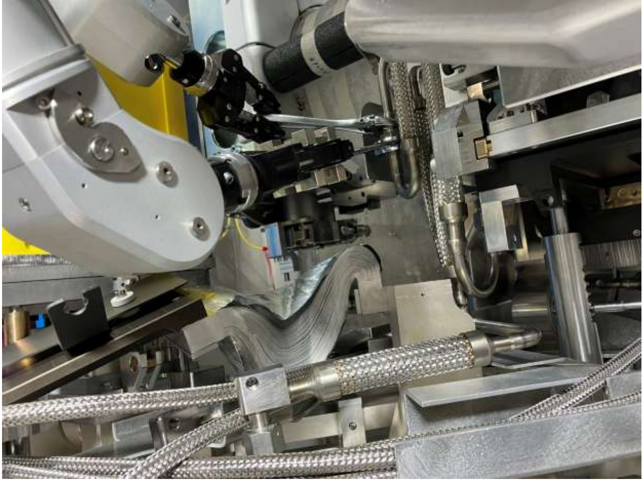
VCR joint re-tightened.
