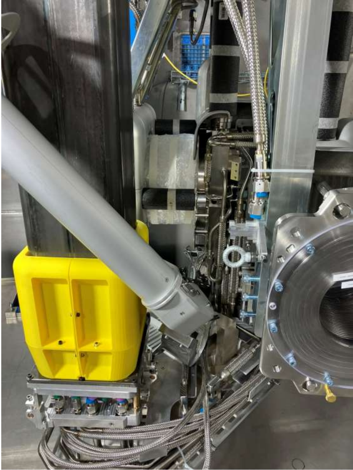
In this orientation, adjustable wrench not able to reach VCR on second to bottom line.
