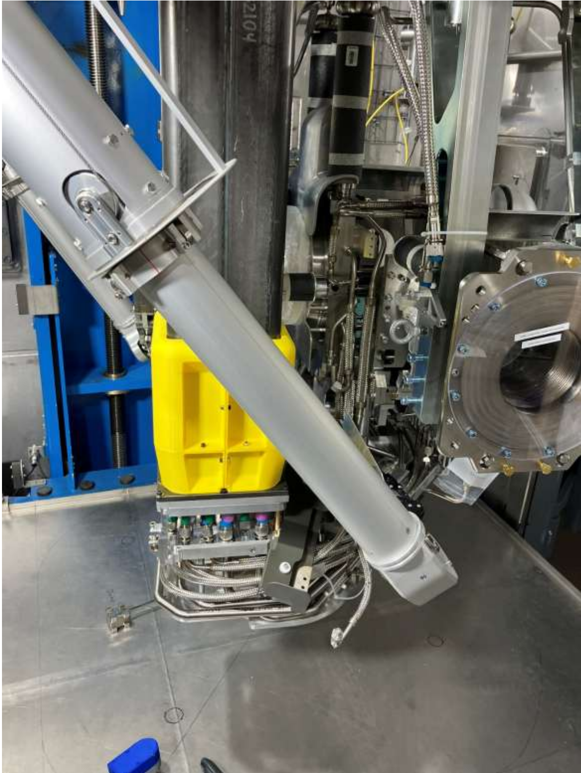
Sheet metal tool used to push the VCR nut up from U-bend
