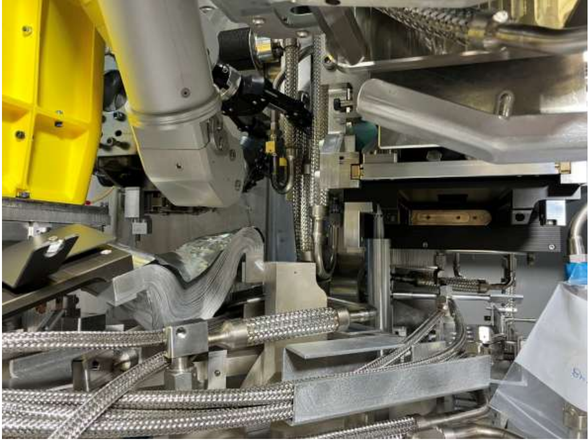
'Pinching' action to position the flexible line and keep the male side from rotating.
