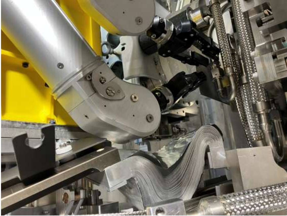
Orientation where VCR nut could be started with the manipulators without too much interference with the HV shield.
