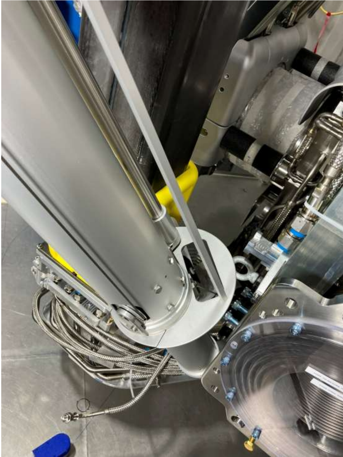
Manipulator arm interference with polished plate assembly
