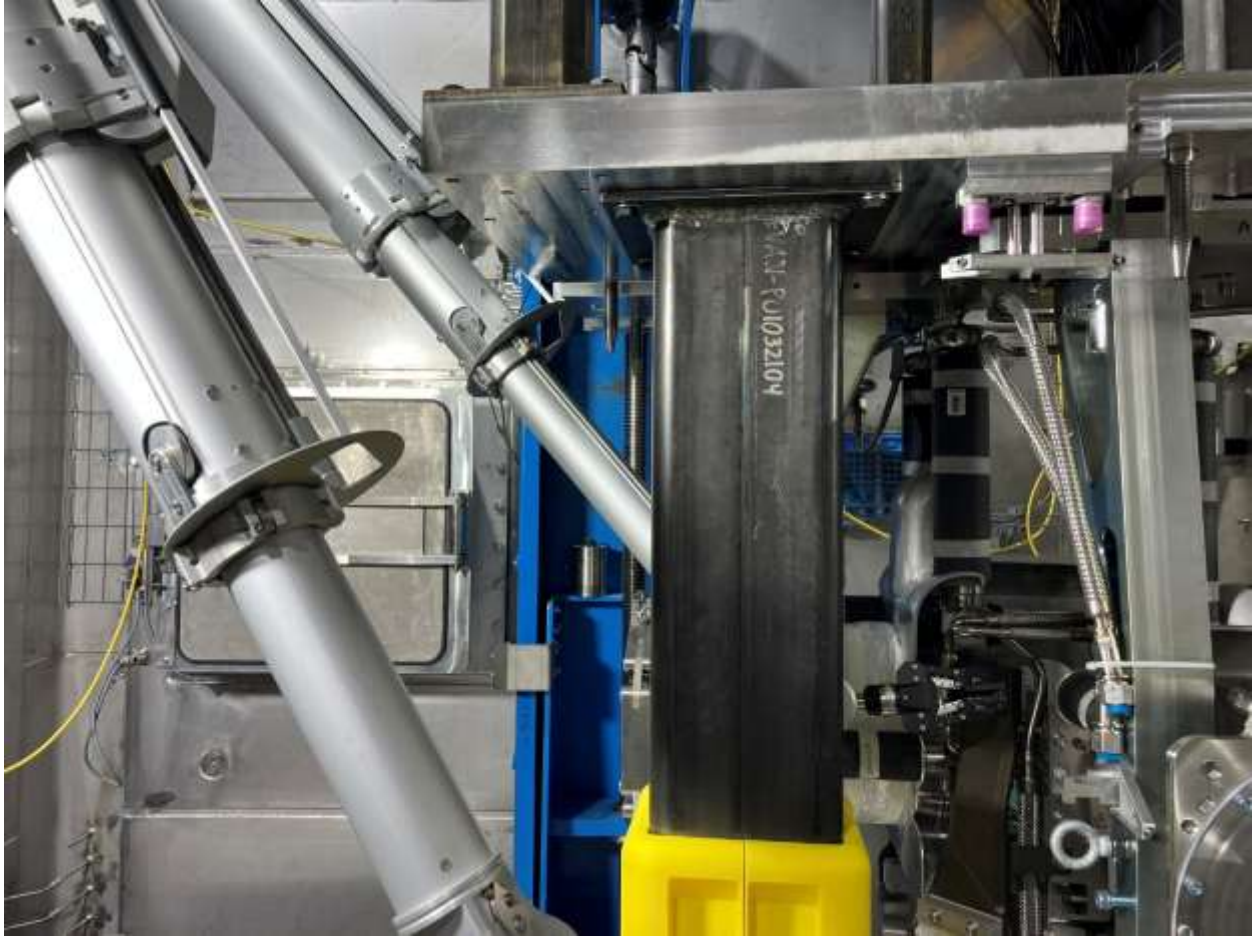
Second manipulator coming in to retrieve busbar screw, minor interference with shielding at the top.
