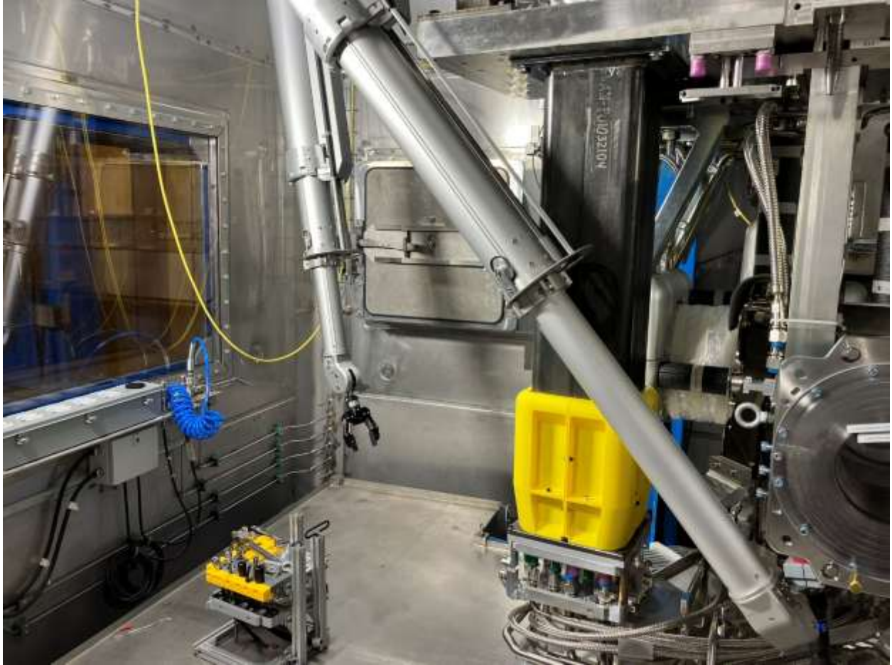
Attempting to reach big screw for the busbar sheet, some interference between manipulator shaft and shielding above
