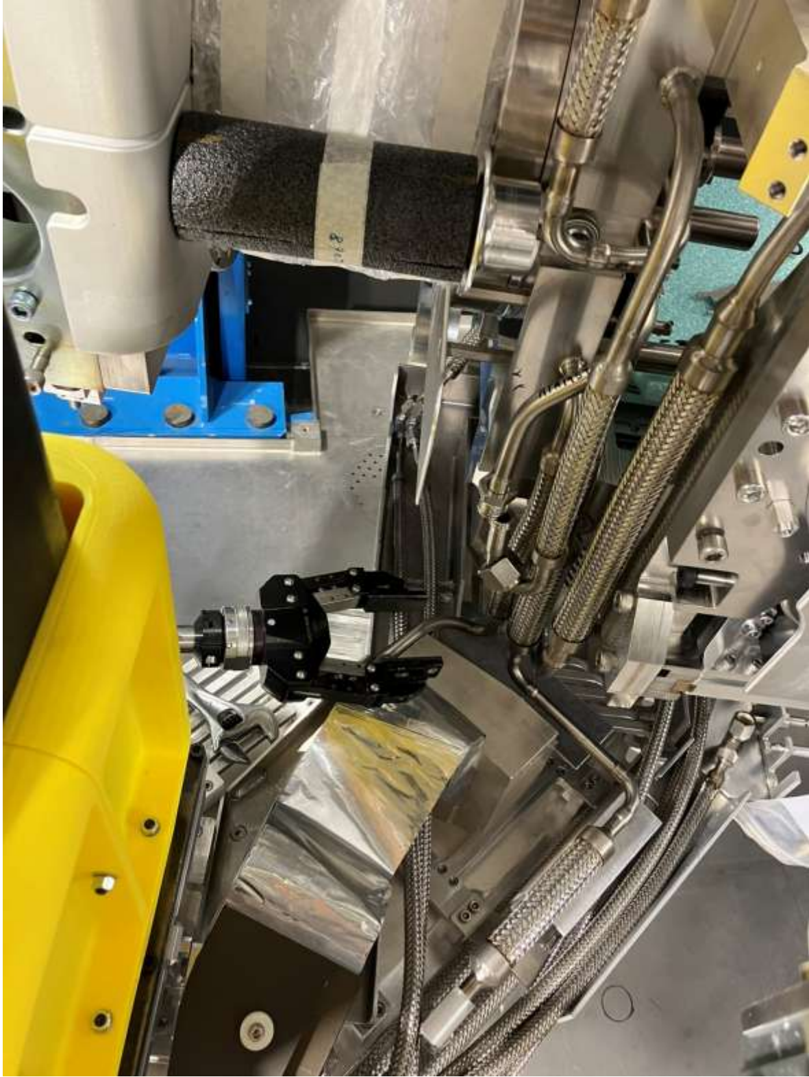
VCR joint successfully seaprated
