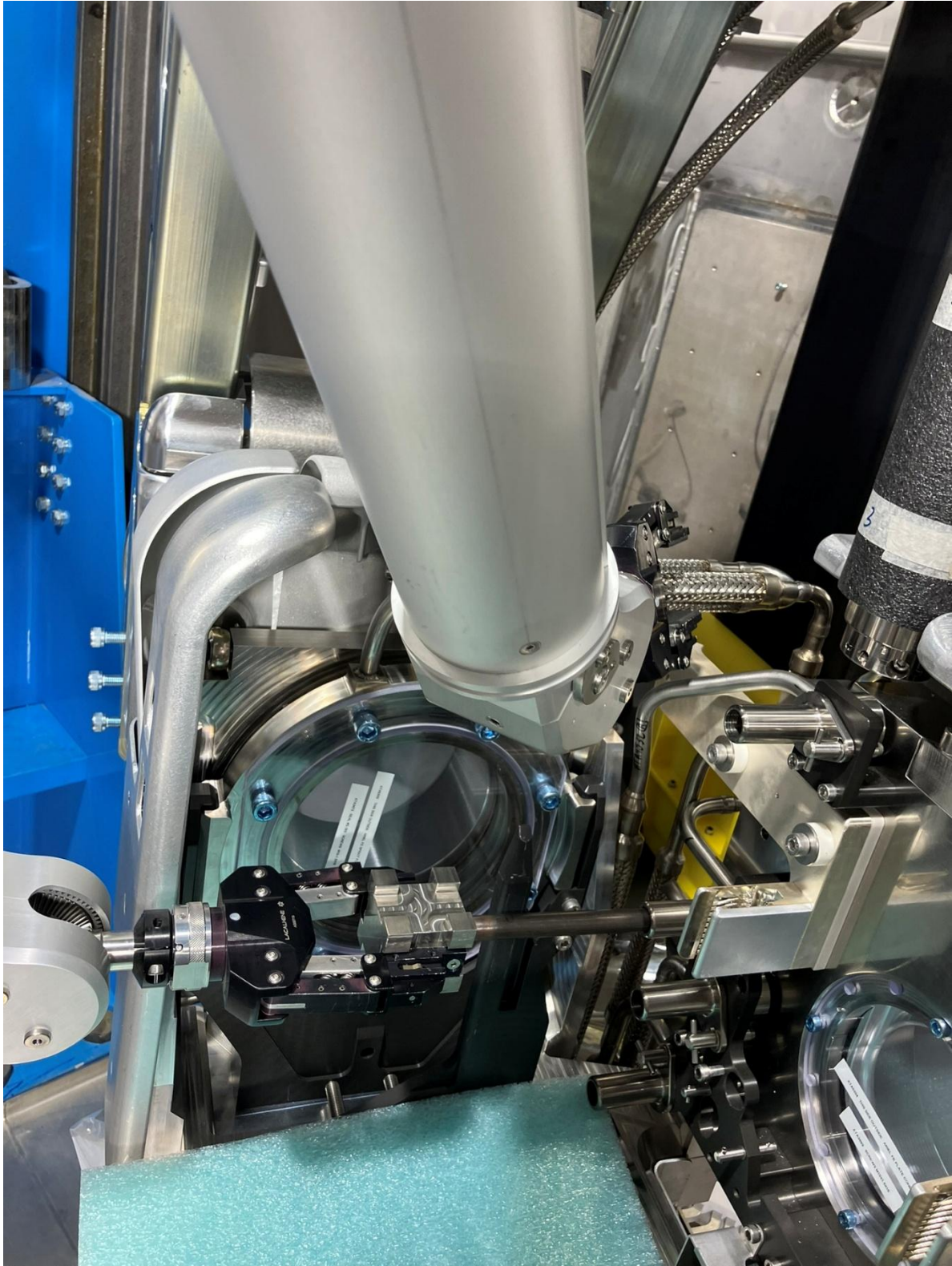
Pin tool interfering with HTV post when using for the second to top line.
