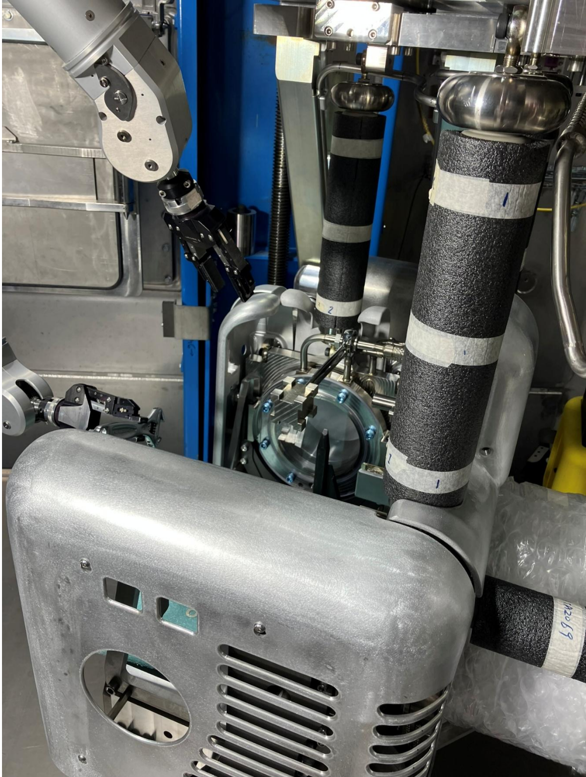
12-point closed wrench on VCR nut.
