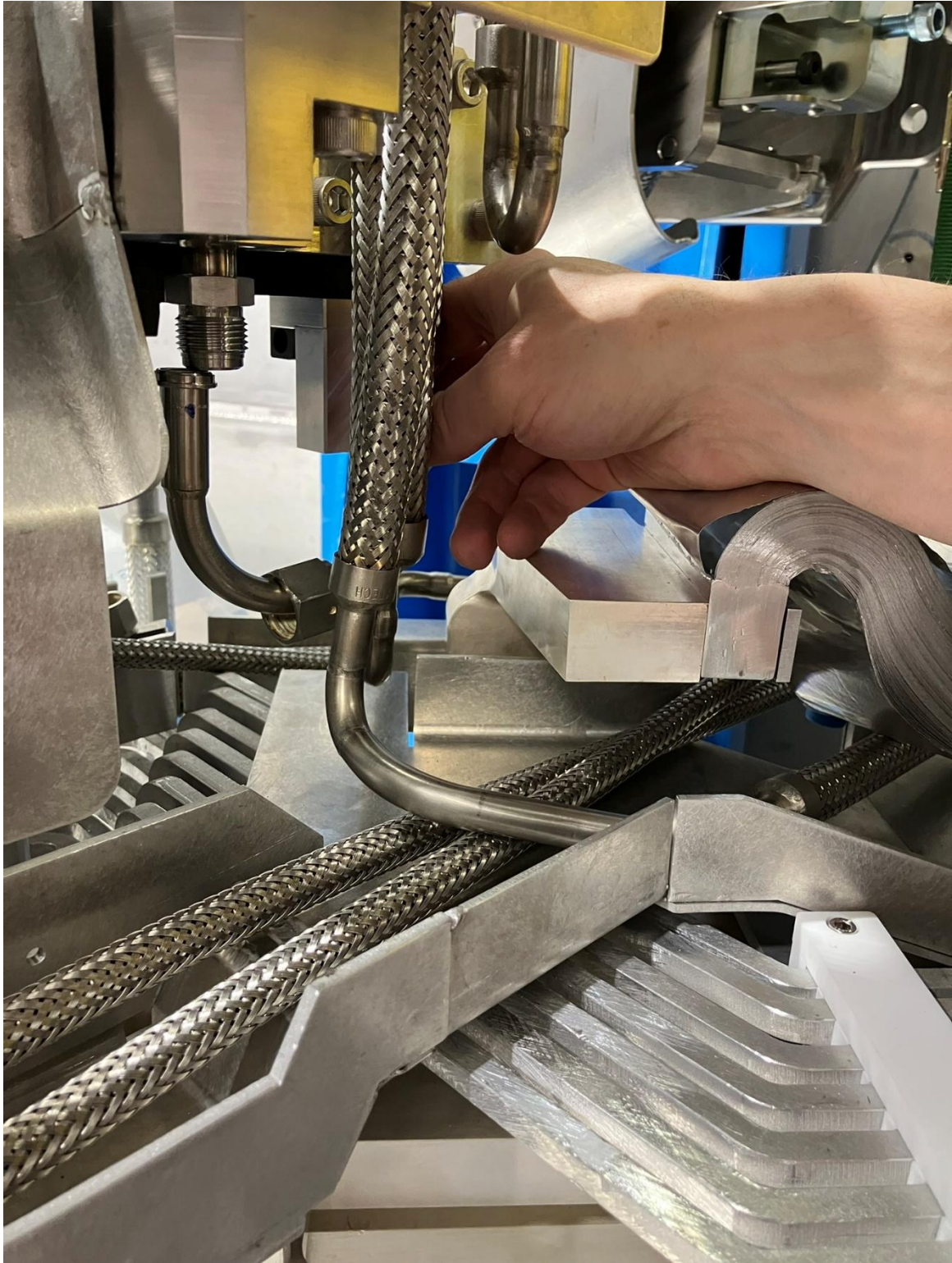
Nut falling in top line's VCR joint 'U' bend.
