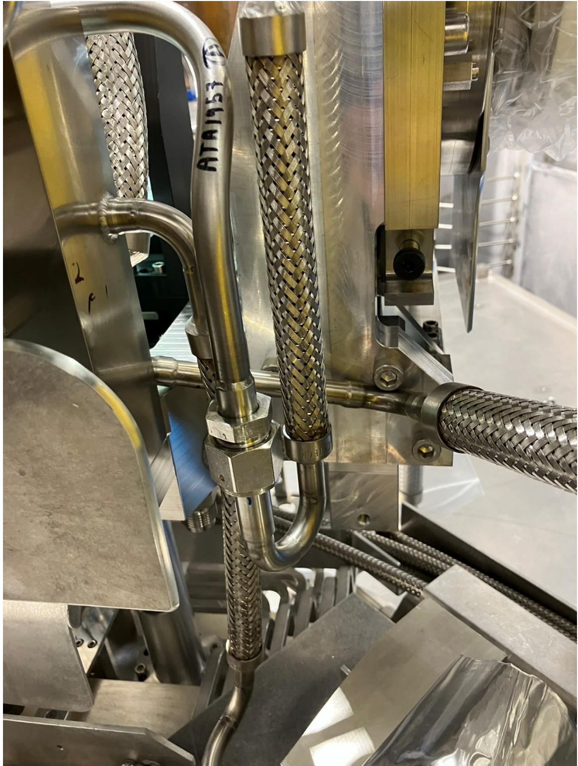
Bottom line catching on screws when returned/removed.
